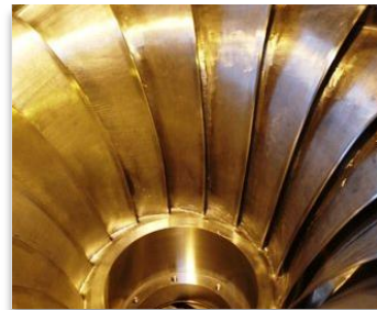
Casting of the francis impeller
