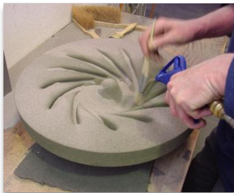
Finishing with air pressure
